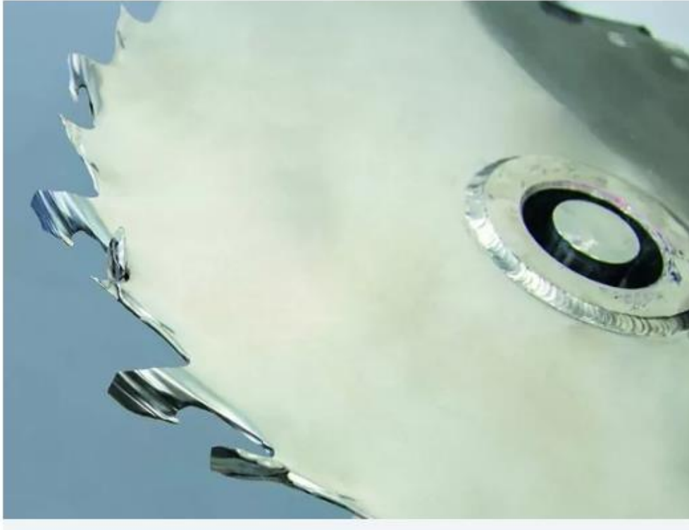
Metal dissolver after 20 hours
