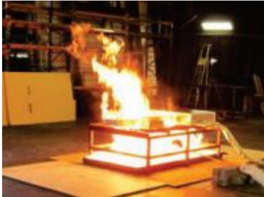
Reg. 100 fire test on SmartBatt pack.
