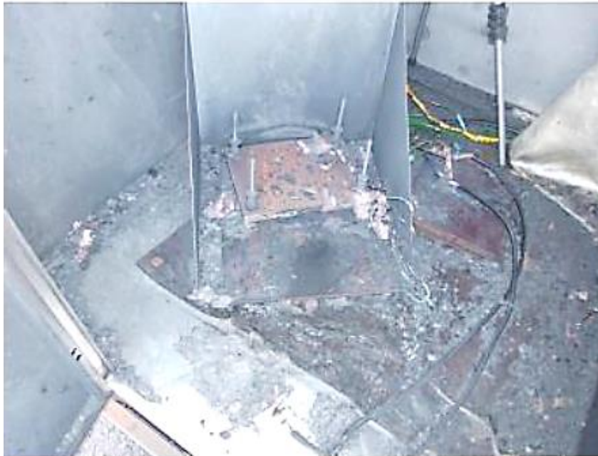
SmartBatt: Failed overcharge test, test passed at cell level but failed at module level, which was not predicted by simulation.
